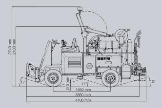
Self-propelled spraying machine **WEIRO® TM 804 SH** with a net capacity of 800 I to ensure the reliable layer bonding with polymer modified binders, i. e. according to TL BE-StB 15 (bitumen emulsion) and tack coat binders, equipped with ROPS (foldable), certified according to DIN EN ISO 3471:2010-01
