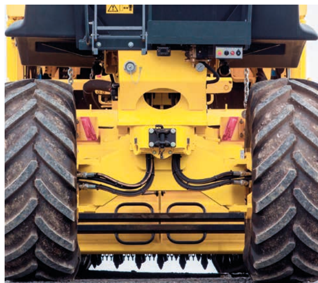
Rear axle with powerful single drives (RS 500).
