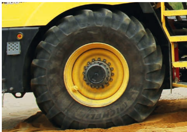
Large wheels for low ground contact pressure.
