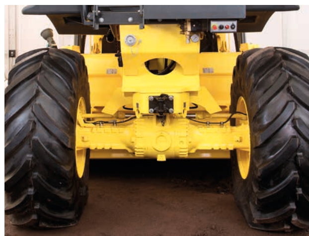
Non-spin oscillating axle \pm 15^\circ (RS 460).
