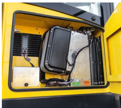
Access to the radiator and maintenance opening for the air conditioning unit.
