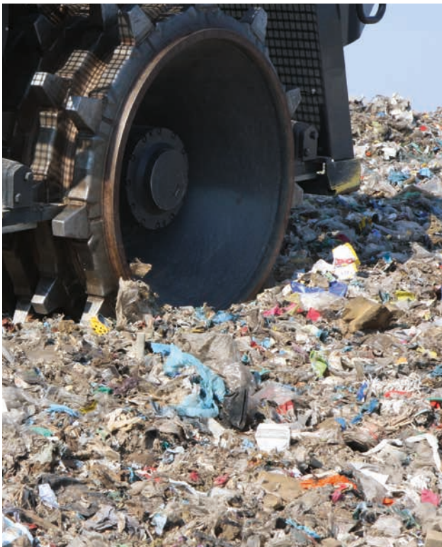
Scrapers ensure clean wheels and high compaction.
