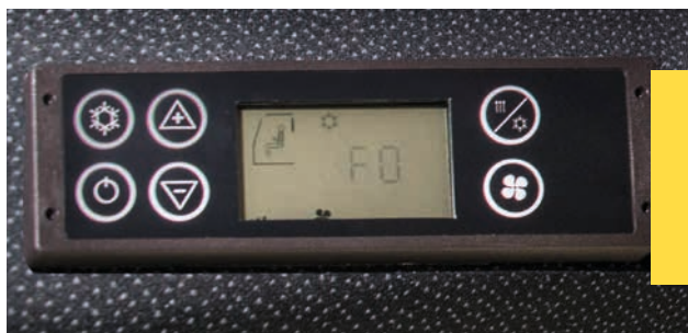
Automatic heating and air-conditioning unit control panel.
