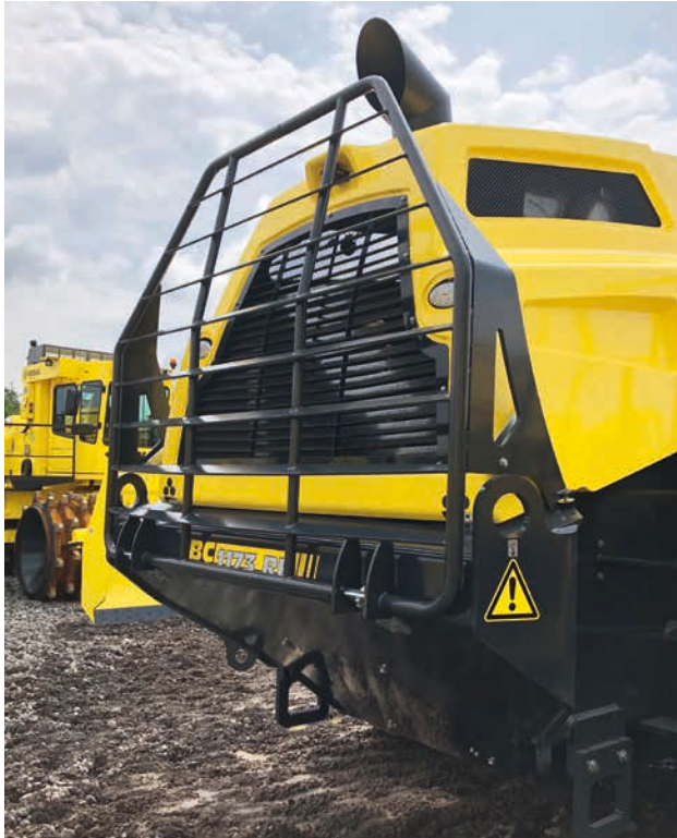
Rear bumper protects the rear of the bonnet from damage.
