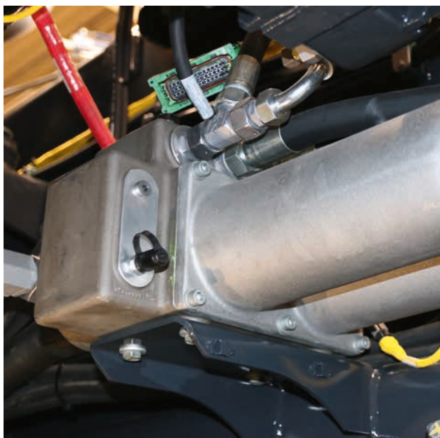
Electronic monitoring of hydraulic return filter.
