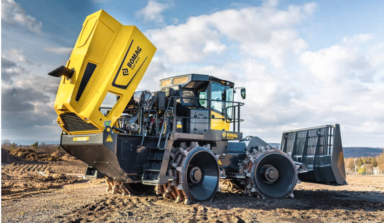
Direct access to the engine – accessible all around.
